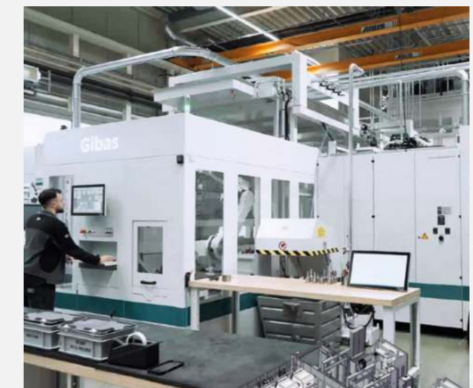
Workpiece robot on five VERSA 5-axis machining centers with rack magazine
