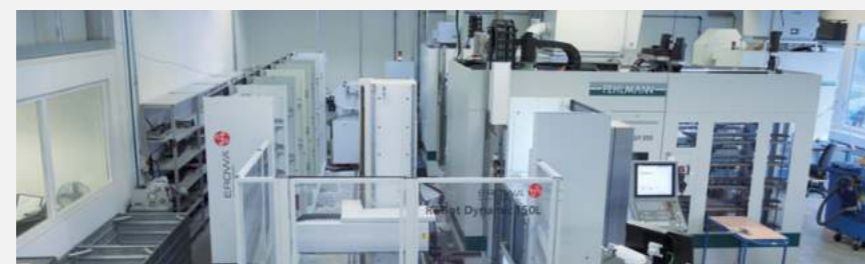
Two VERSA 5-axis machining centers with modular robot system Erowa Robot Dynamic 150L
