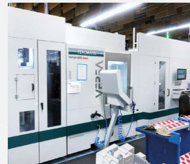
Two VERSA 5-axis machining centers, each with a rack magazine with a robot-assisted parts handling system
