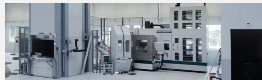
VERSA production island 5-axis machining center with rack magazine, articulated arm robot for parts handling and high-bay storage for raw and finished parts
